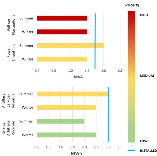
Figure 2-12 Mueller ESS sizing by use case summary
