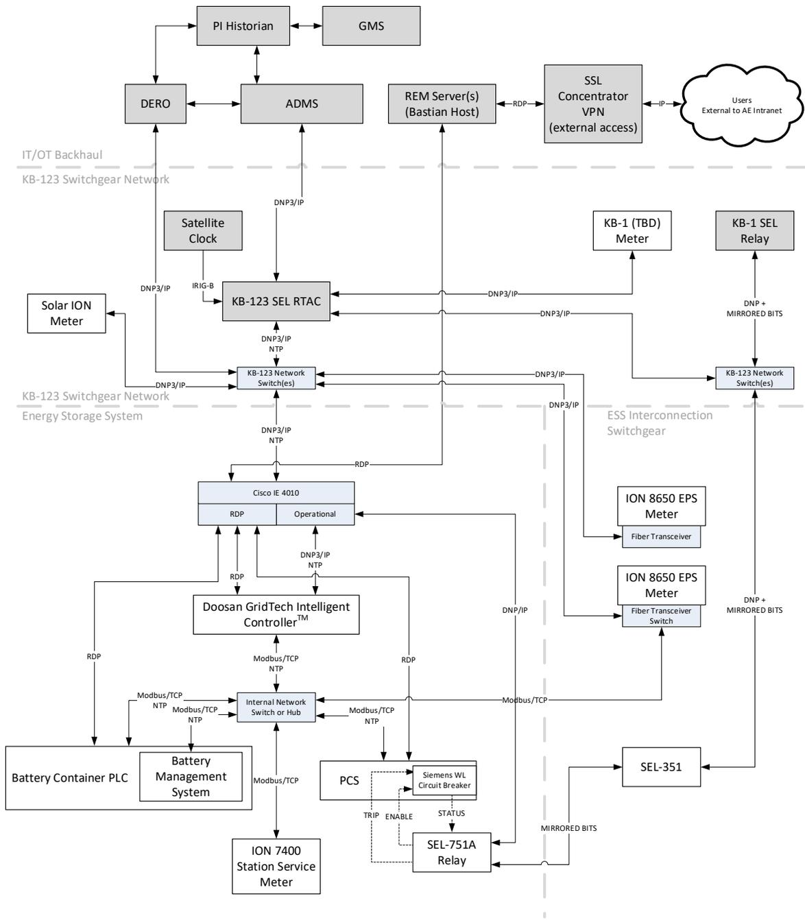
Figure 2-13 Kingsbery ESS communication paths and control architecture
