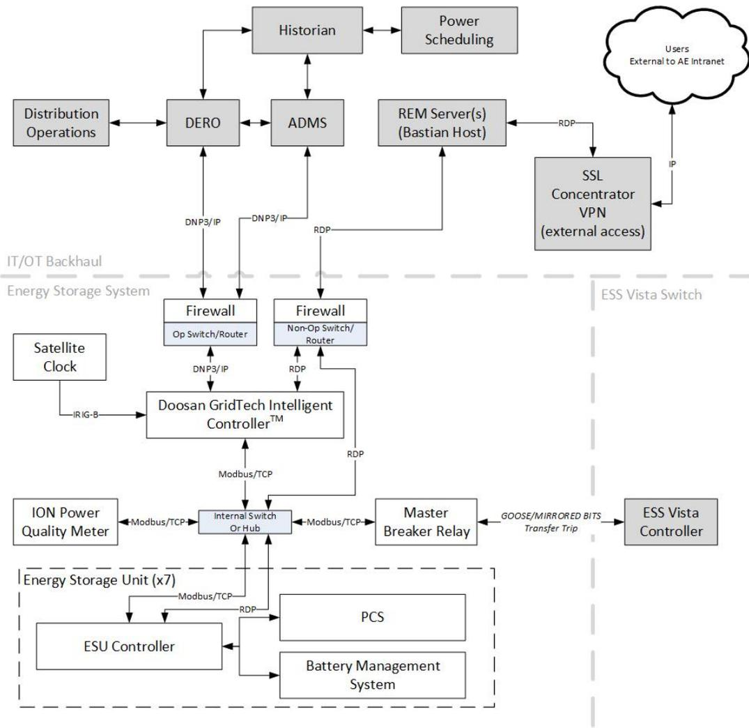
Figure 2-14 Mueller ESS communication paths and control architecture
