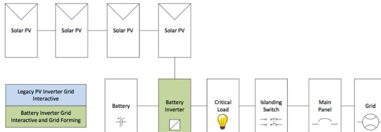
Figure 4-1 Energy Storage System Block Diagram DC-Coupled
