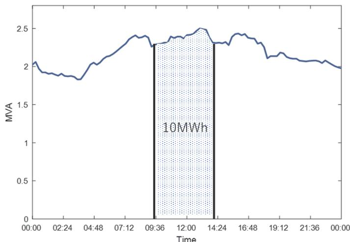
*Figure 2-6 Outage ride through energy capacity requirement*
